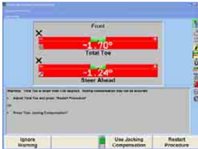
Total Toe is larger than the preset tolerances.
