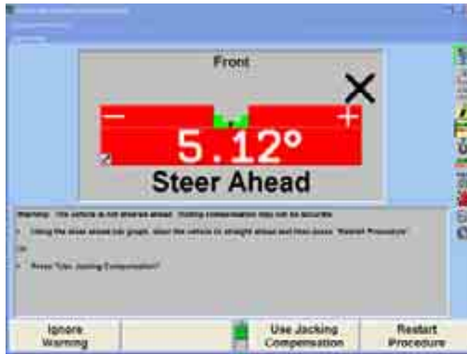
The vehicle is not steered ahead.
